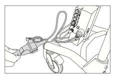
Battery charging must take place when the walker is not in use (the battery can never be overcharged). Charging is carried out by inserting the plug in a wall socket.
